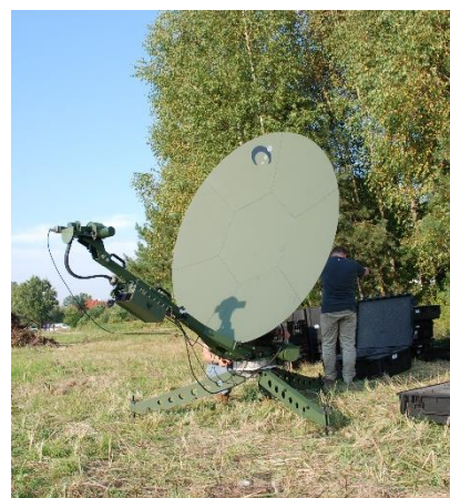
Fig. 6 SMART - terminal with offset dish parabolic antenna
