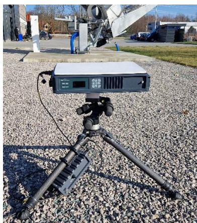
Fig. 4 Phoenix - terminal with a flat panel terminal antenna
