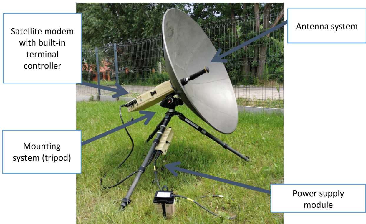
Fig. 1 SatPack COBALT - the flagship representative of the Manpack class, modular backpack terminals
