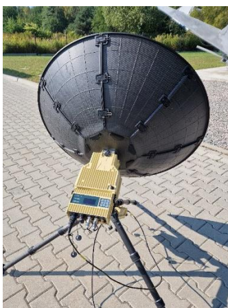
Fig. 5 SatPack COBALT - terminal with central feed parabolic antenna.
