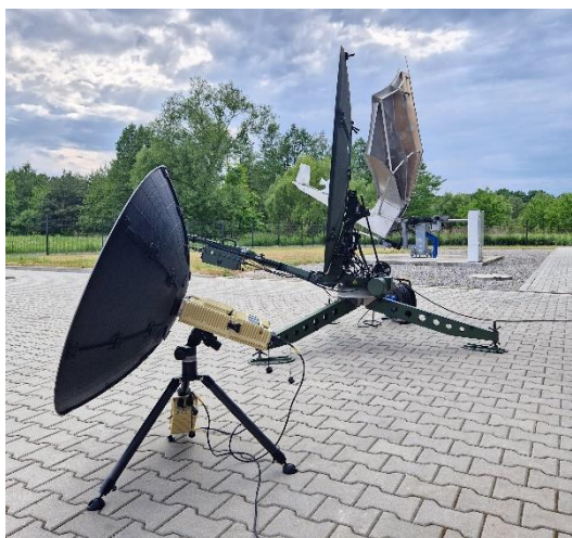
Fig. 2 Terminals designed for operation using GEO orbits - SatPack COBALT, SMART, HUB-Master station
